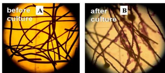
Fig. 1: Optical microscopy images of the carbon fiber felt before (A) and after (B) depositing of microorganisms.
